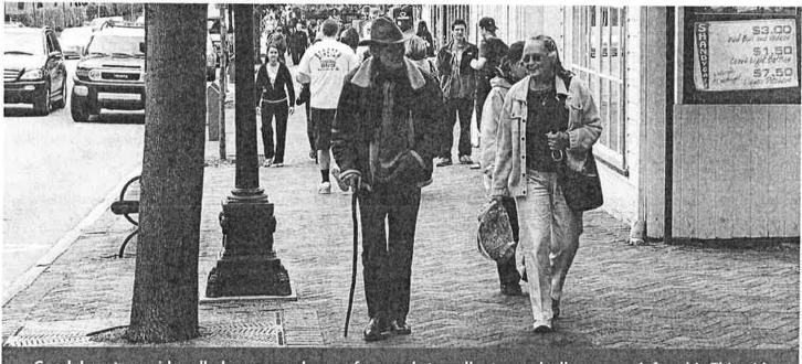
Good downtown sidewalks have enough room for people to walk, stop and talk, or even sit for a bit. This wide sidewalk in State College, Pa., is made of visually appealing paver stones. Care must be taken when installing paver and similar surfaces so wheelchairs and other wheeled devices can roll smoothly over them.
